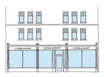
By dividing the shopfront into 3 symmetrical bays proportionately the shopfront relates much better to the upper floors. The stallriser, pilasters and cornice ground the shopfront and provide it with a more solid frame and structure. The fascia is much better proportioned and respects the rhythm of the building.
