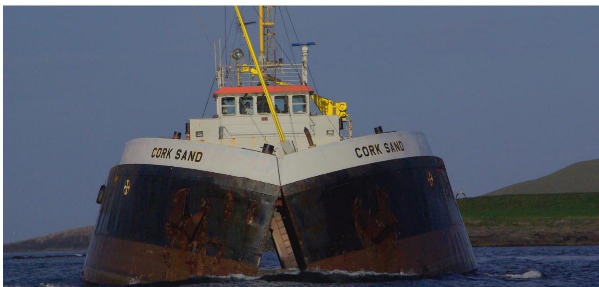
Photograph 3-1 Example Hopper and Transportation Barge: Cork Sand (Source: Boskalis 2012)
