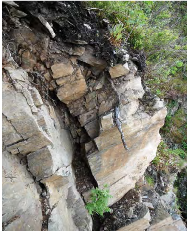
Photo 1: AA7 - 5m 3 detached block with a 150mm dilated release joint.
