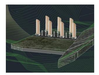
A new headwall and security/debris screen is also being installed at the Culloden Centre. The new screen meets current design standards and prevent blockages of the culvert inlet whilst allowing safer and easier maintenance of the screen.
