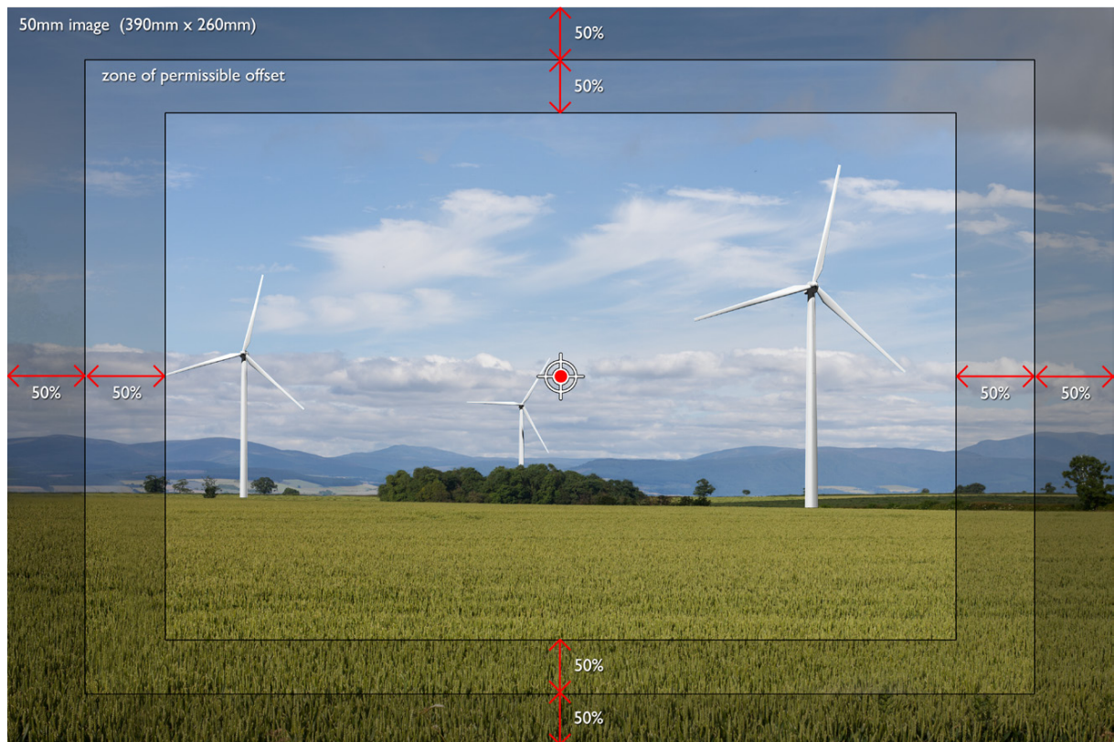
Fig. 11. Image showing the framing of the 75mm focal length and the degree of permissible offsets when recalibrated from the original 50mm photograph. An A3 template which can be printed as a transparency is downloadable from the Council's Planning Guidance and Advice web page.
