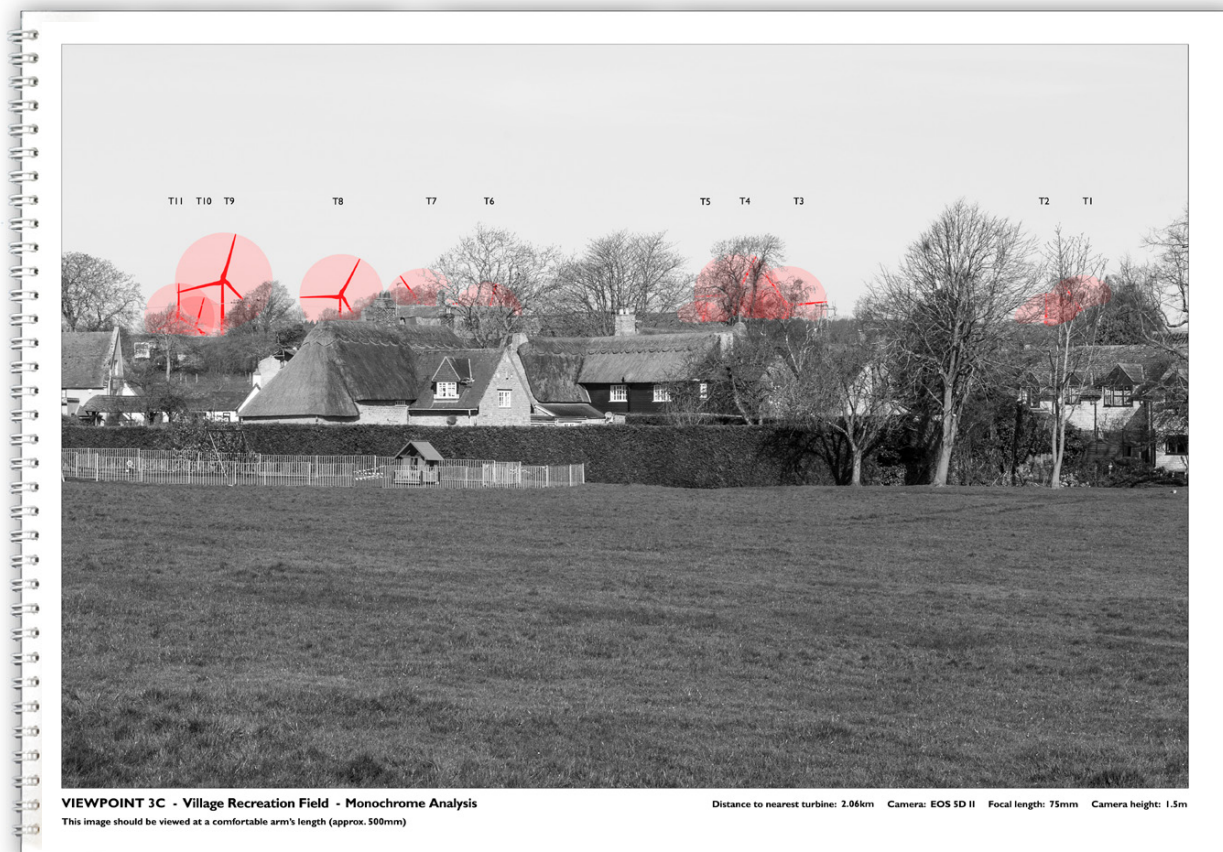
Fig. 13. The blade sweeps shall exclude any landform or permanent structures but not trees or vegetation.
