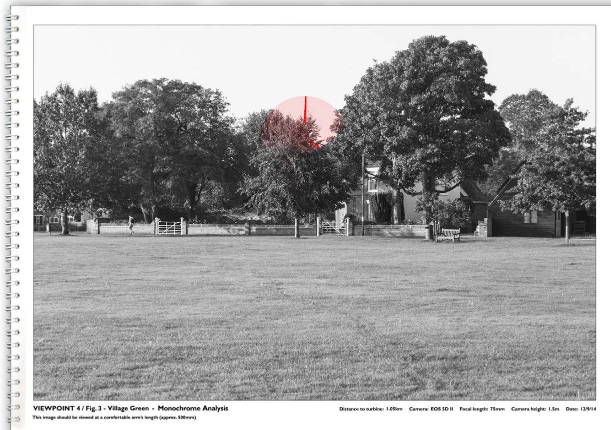
Fig. 18. Where the turbine is screened by trees or other obstructions, the blade sweep shall be shown on a monochrome background and exclude any landform or permanent structures but not trees or vegetation.
