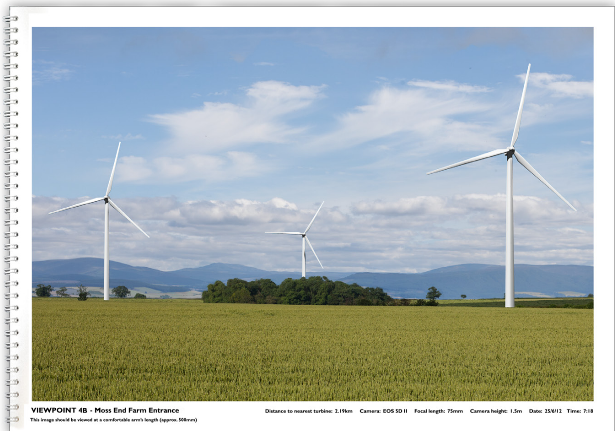
Fig. 12. A 75mm photomontage showing the technical information bar and viewing instructions. The technical information bar below the 75mm image shall contain the same information contained in 4.8, but with the viewing instructions to read: 'This image should be viewed at a comfortable arm's length (approx. 500mm)'
