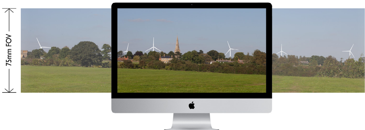
Fig 19 Example of a 65.5° panoramic photomontage. When viewed on a computer screen, the mouse can be used to pan the image which has a similar effect to turning the head to view the wider landscape. The correct focal length is maintained across the overall horizontal field of view.
