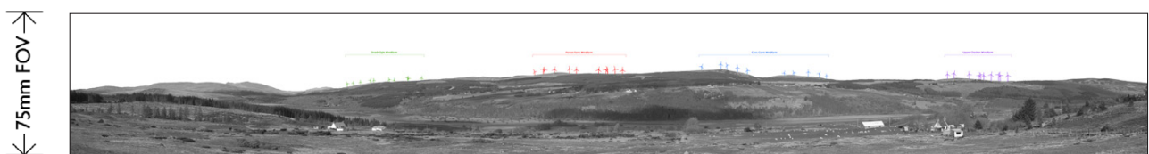
Fig. 21. A monochrome panorama with a vertical focal length of 75mm ( 18.0^\circ ) and a horizontal field of view of 100^\circ .
