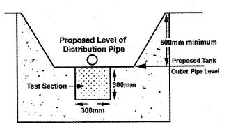
For safety reasons, holes deeper than 1.2 metres must be shored for safe access
