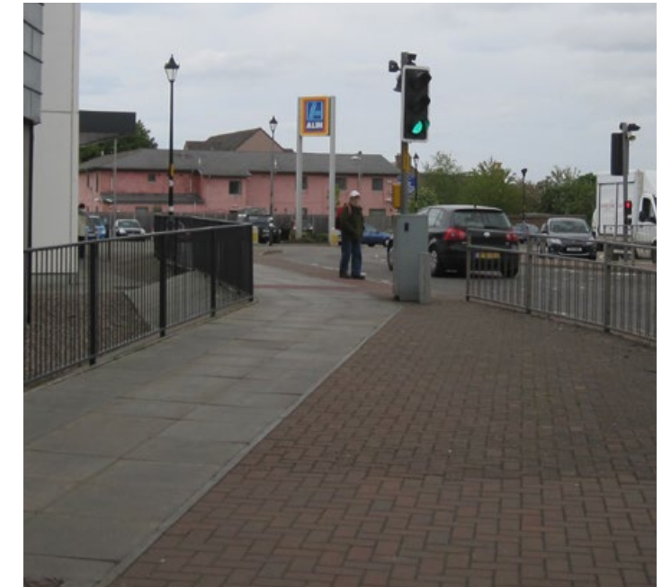
Simple footway (although broken bond slabs look better) but unfortunate use of 'low maintenance' hardscape where grass or soft landscape would be more appropriate.
