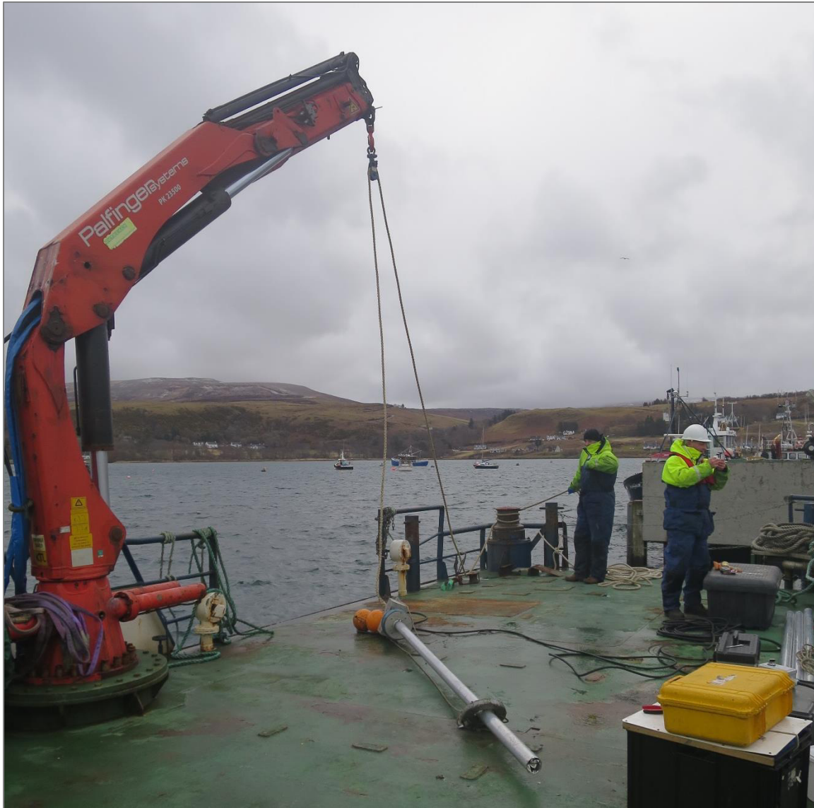
FIGURE 2 - SDI D-4 VIBROCORER AND CORE ON DECK OF JOHANNA G
