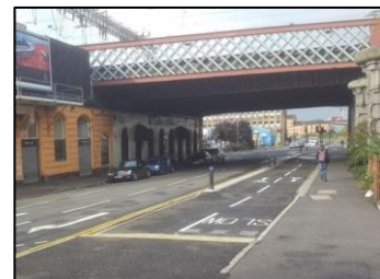
Figure 4-6 - Segregated Cycleway – Two-way, Glasgow
