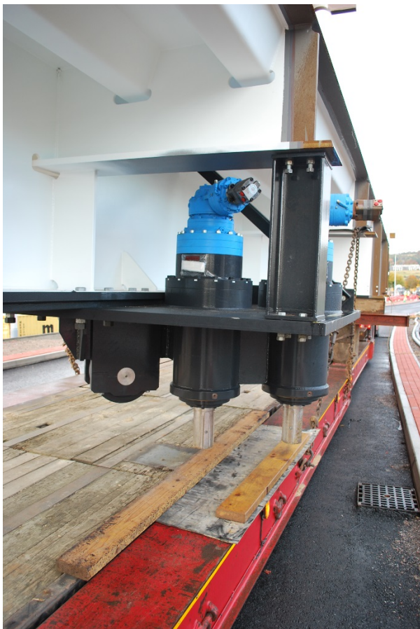
The 2 motors and gearboxes that will rotate the new bridge with the idle wheel to the left of the motors
