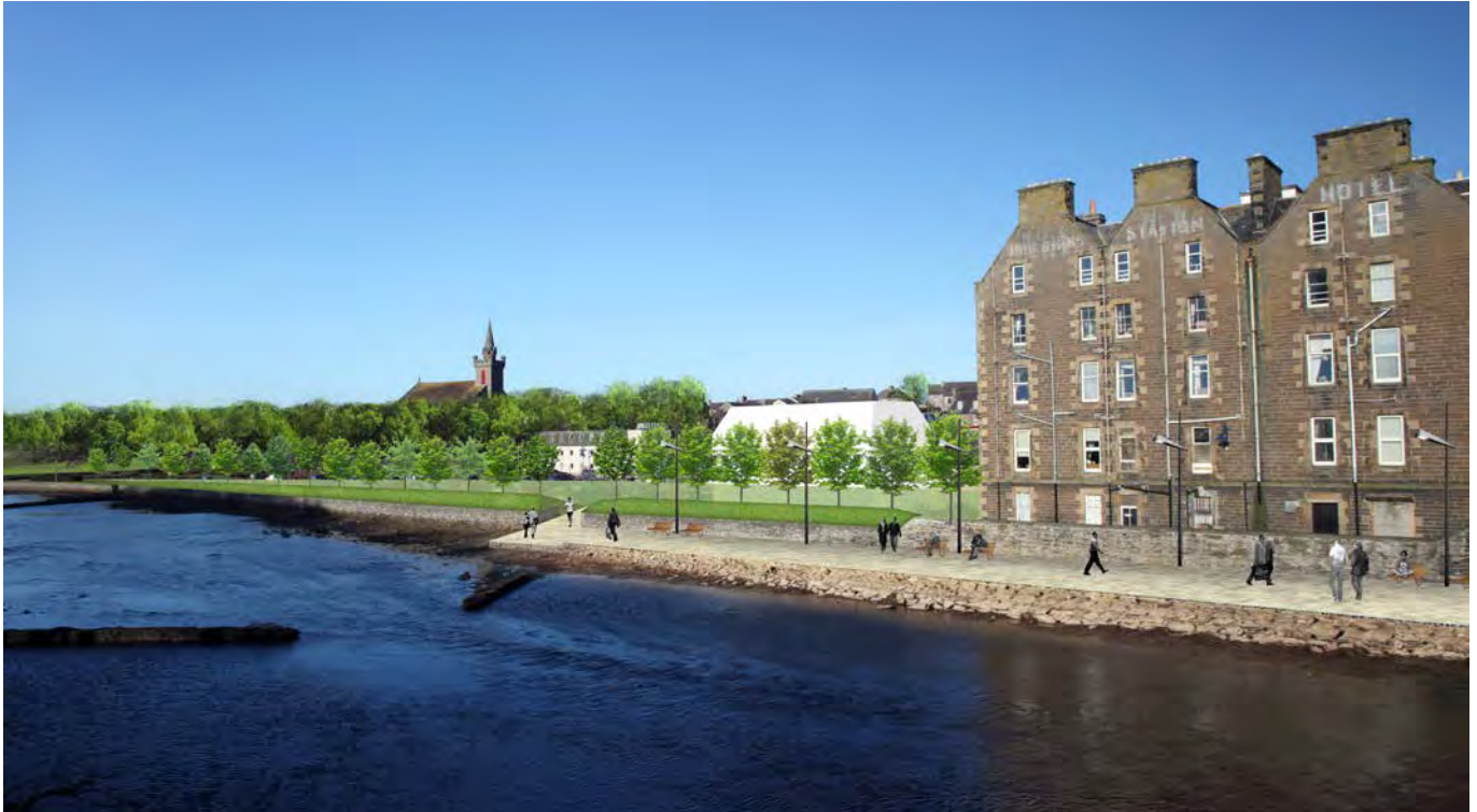
Vision of the new landscaped bund along the river edge to mitigate flooding,
