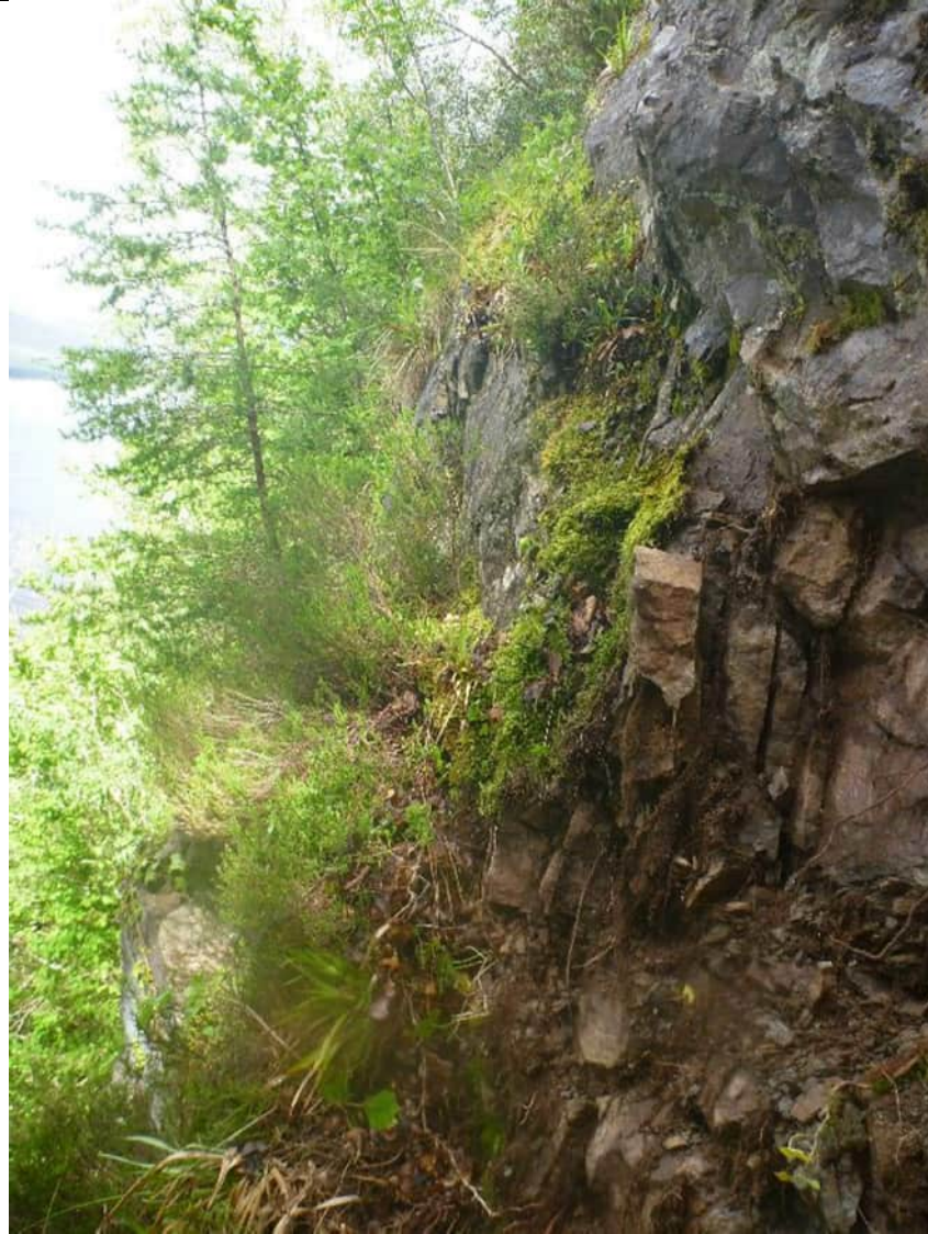
Photo 10: Weathered rock mass at failure source at mid to lower portion of upper crags.
