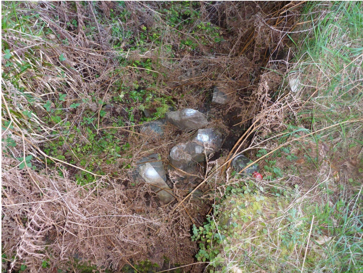
At Ch. 390 - Several blocks up to 0.4m x 0.3m x 0.2m in ditch. Source not obvious.
