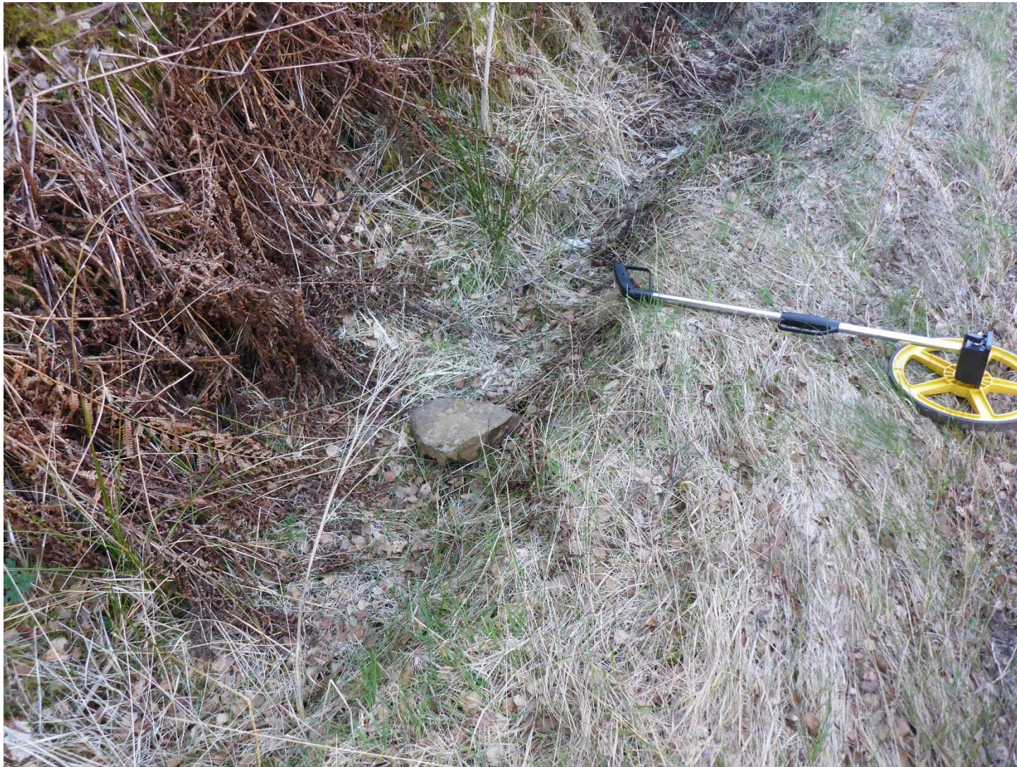
At Ch. 3870 – recent block fall in 2023 (planar failure). Block c.0.1m x 0.1m x 0.1m in ditch.
