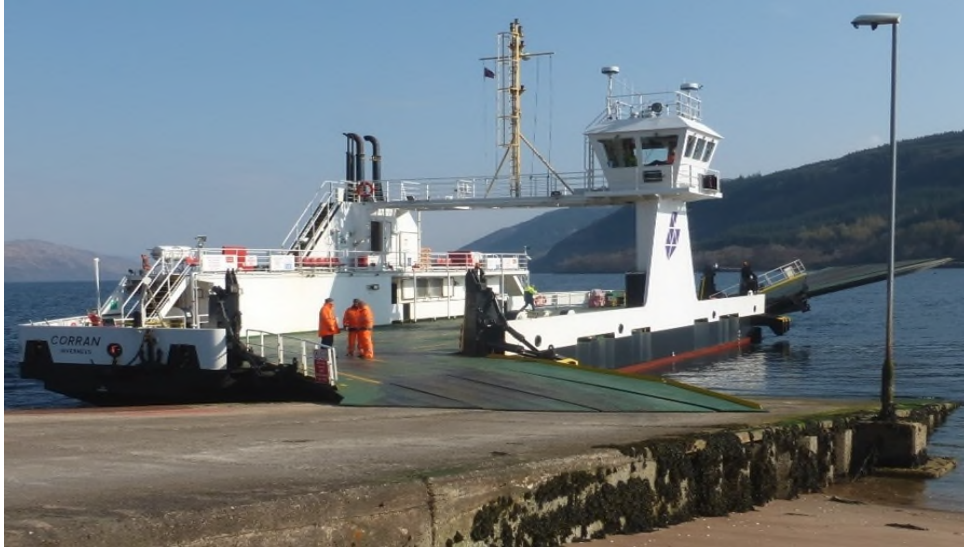
Figure 3.2.2: The MV Corran Quarter-point Loading Vessel on the Ardgour Slipway
