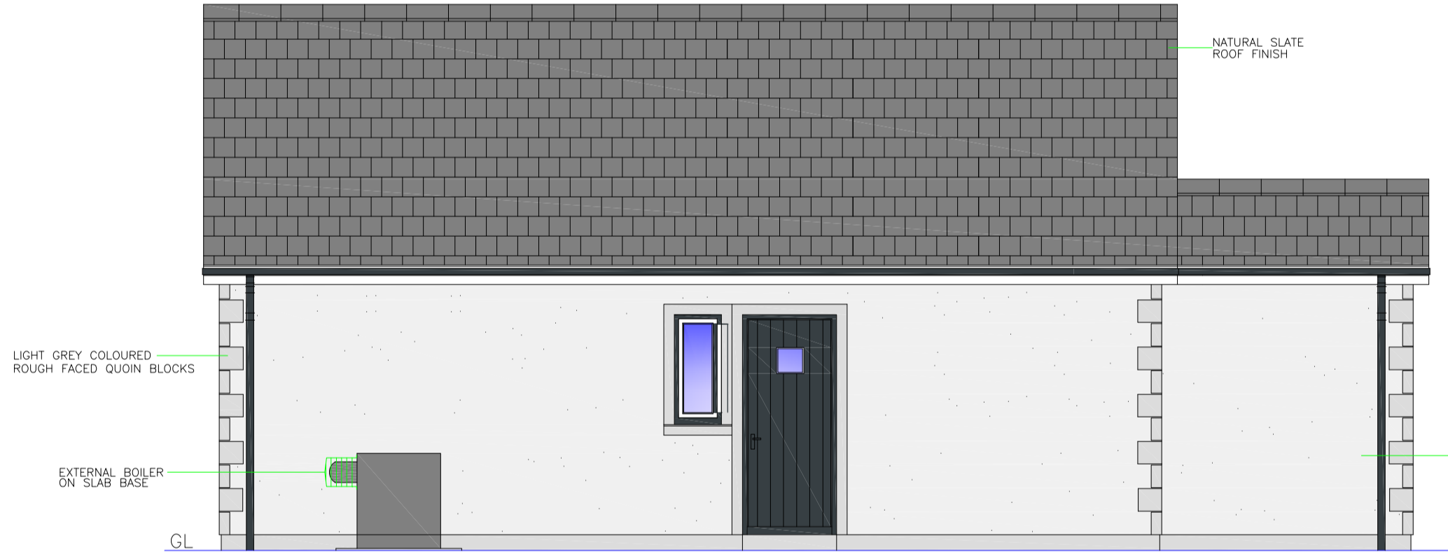
North East Elevation 1:50 Facing 11 Ness Way
