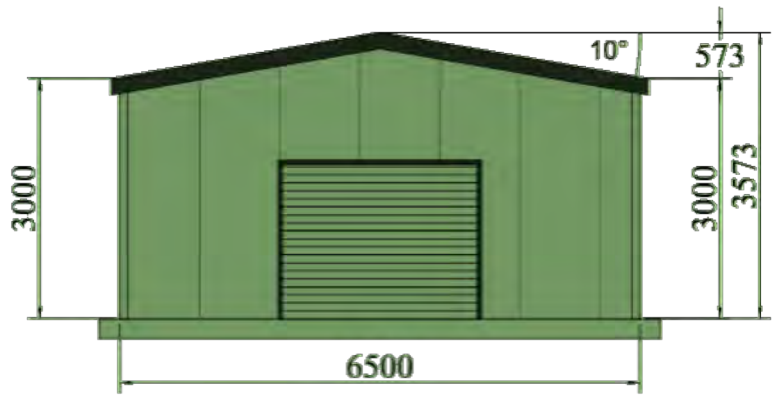
Front Elevation (External)
