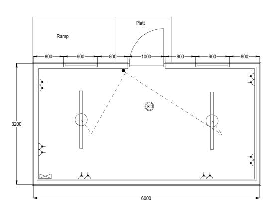
Extension to be wired to 17 edition IEE regulations Power supply 2.5mm T&E Light Circuit 1.5mm T&E wiring taken bak to existing consumer unit
