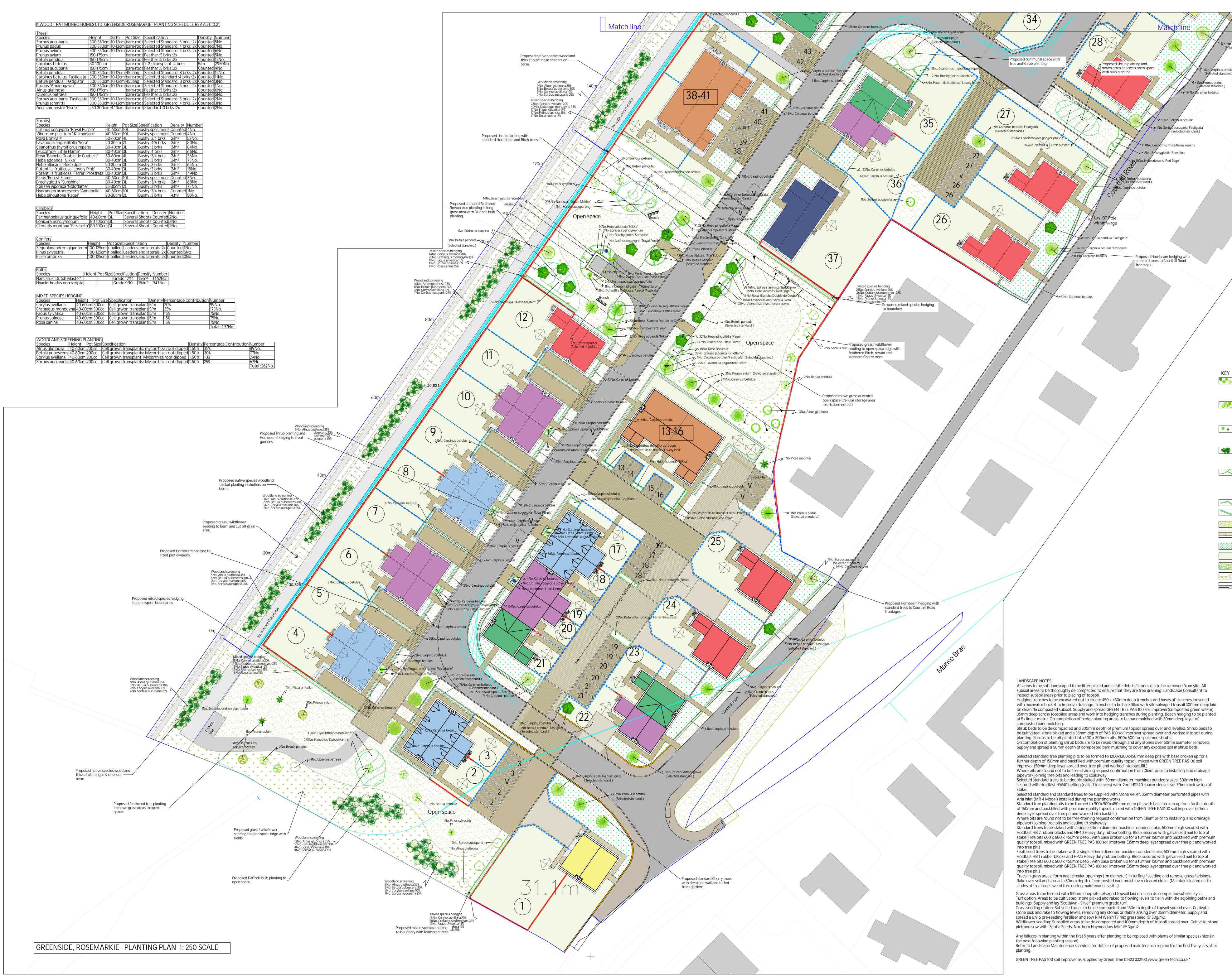
Proposed 3.0-3.5m tall, 10-12cm girth selected standard tree planting- trees to be pit planted into 1.2m diameter x 450mm deep prepared tree pits. Base of tree pits to be broken up for a further depth of 150mm. (Reform neat circles , 1.2m diameter at tree bases in grassed areas.) Birch, Hornbeam, Cherry and Rowan species.
