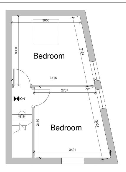
Second Floor Plan Scale 1:50 Floor area = 23m<sup>2</sup> Key: Heat = Heat detector ION = Smoke detector CO = Carbon Monoxide detector FE = Fire Extinguisher FB = Fire Blanket
