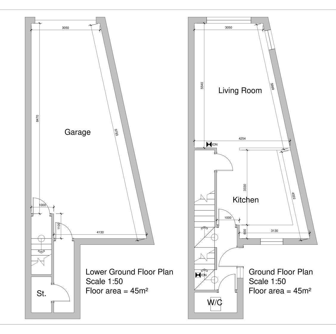
Key: Heat = Heat detector ION = Smoke detector CO = Carbon Monoxide detector FE = Fire Extinguisher FB = Fire Blanket
