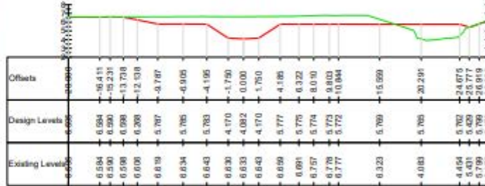
CH 430.000 m Natural scale - Looking downstream
