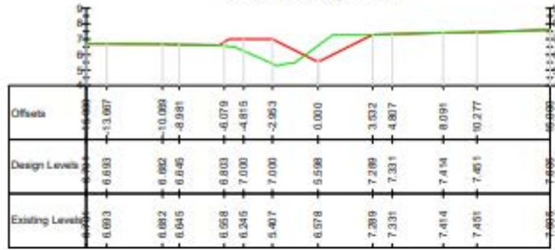
CH 25.000 m Natural scale - Looking downstream
