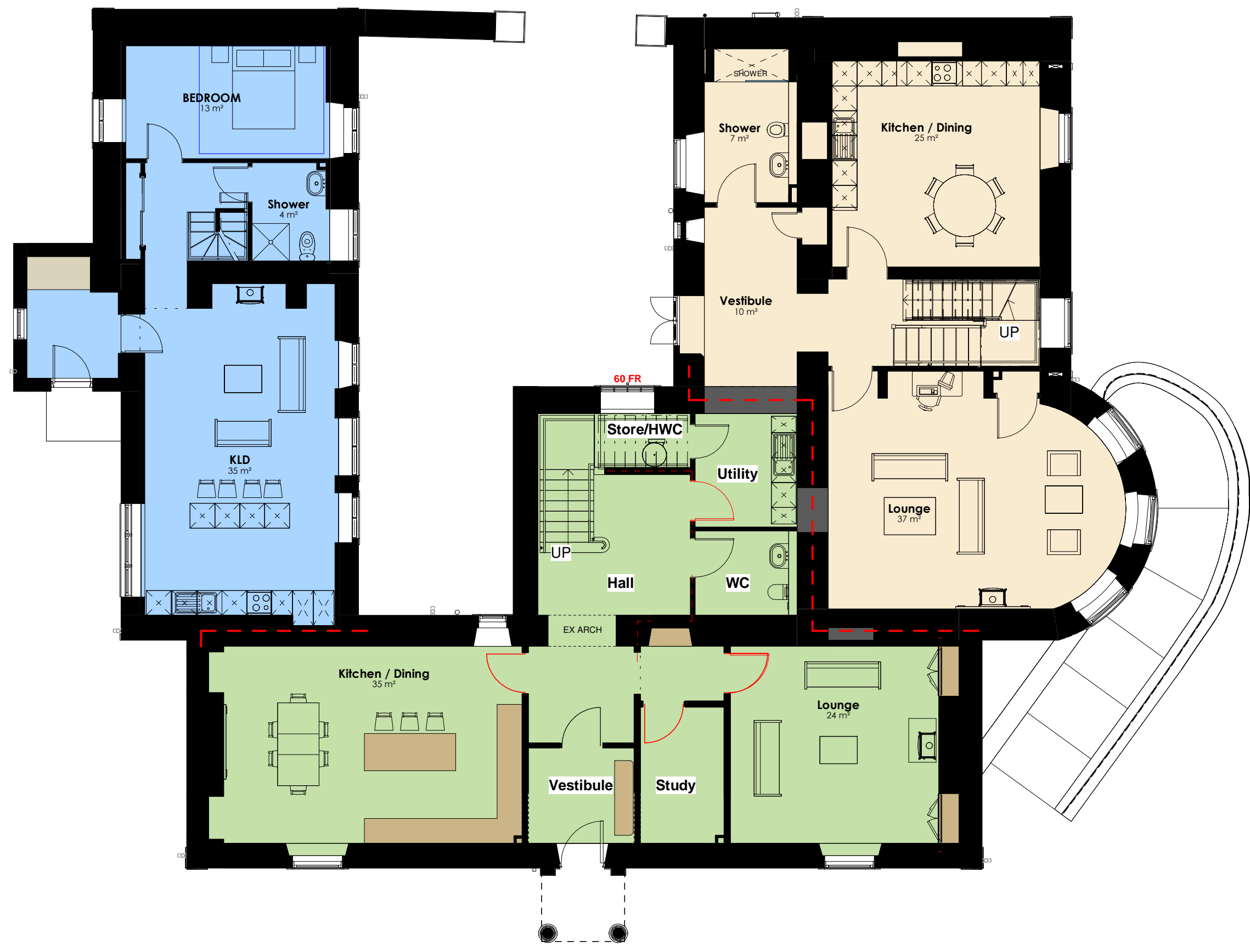
00-Ground Floor Plan - Proposed O/A
