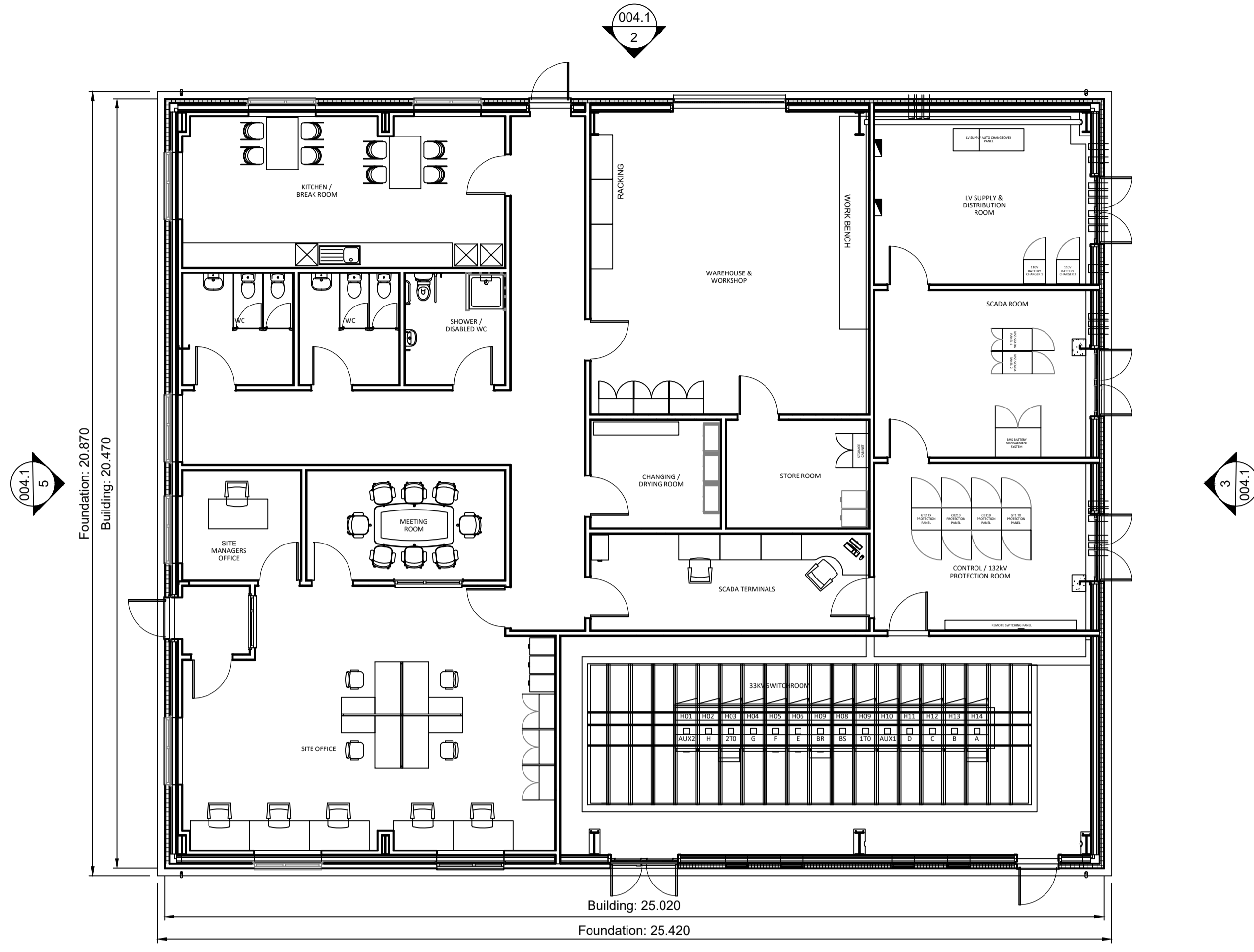
1 Substation Building Plan Scale 1:100 @ A1
