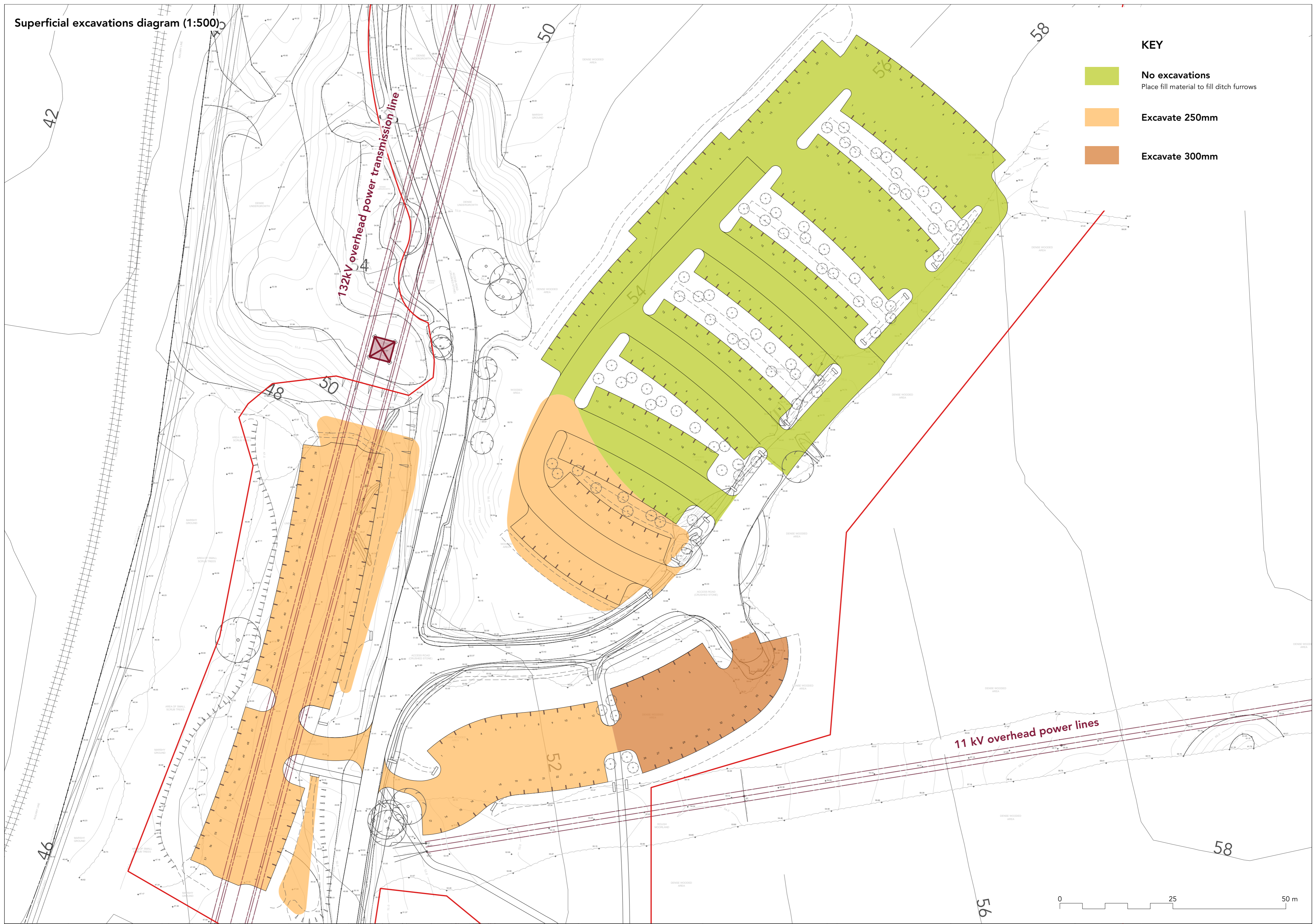
Cut & fill diagram (1:500)
