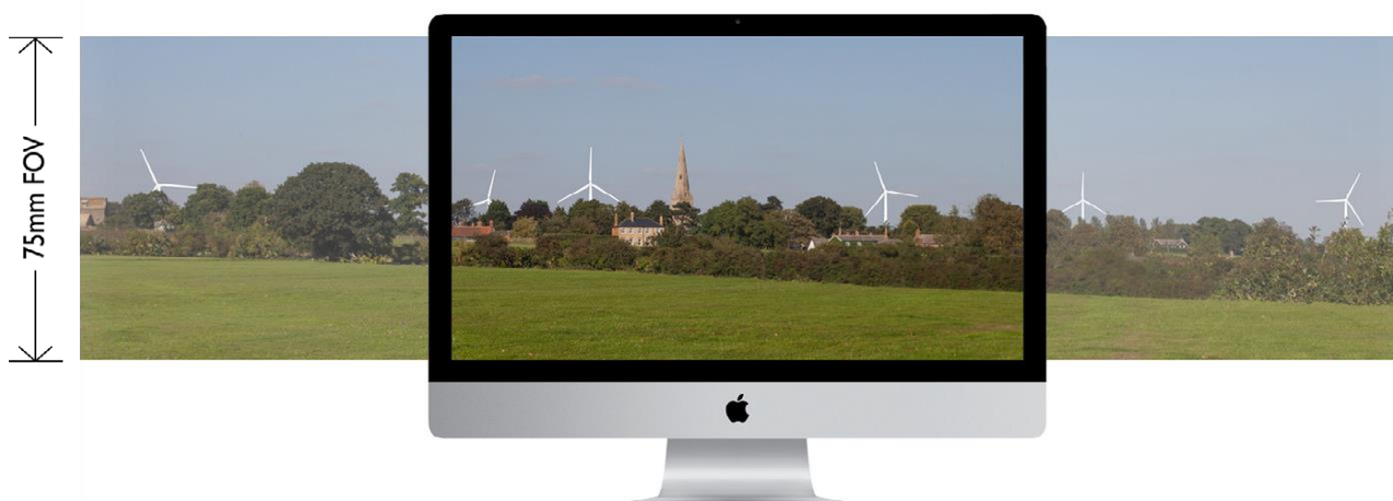
Fig 19 Example of a 65.5° panoramic photomontage. When viewed on a computer screen, the mouse can be used to pan the image which has a similar effect to turning the head to view the wider landscape. The correct focal length is maintained across the overall horizontal field of view.
