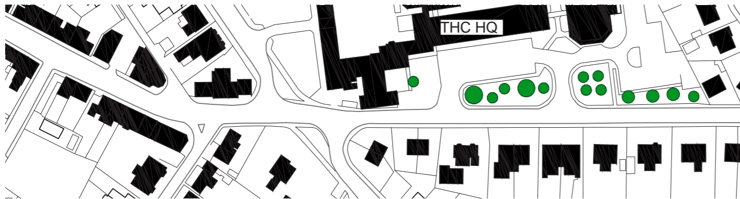
Glenurquhart Road / Tomnahurich Street figure ground diagram THC offices set back but enclosure maintained by street and in-curtilage trees. Tomnahurich Street, buildings tight to back of footway, urban enclosure, about 1:2.5
